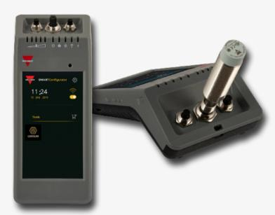
The SCTL55 Series IO-Link Smart Configurator provides a means to configure most IO-Link sensors with a wireless device that replaces the need to program via a USB IO-Link Master connected to a PC or via a network connected master device. The only thing required is the IO-Link Smart Configurator.
