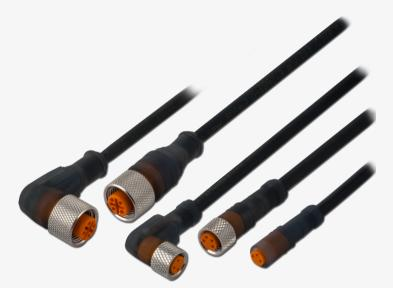
The M12 and M8 CONB Series cordsets are available with a straight and 90 degree angle connector for three, four or five conductor sensors. They come with two, five, ten or fifteen meter standard PVC jackets. For more harsh environments, they are also available with 100% PUR jackets. PUR is more flexible and durable than PVC, it is also tear-resistant, abrasion-resistant, and provides improved resistance to coolants, oil, and grease.
