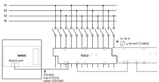
Fig. 11 Three-phase system with neutral (4-wire).
