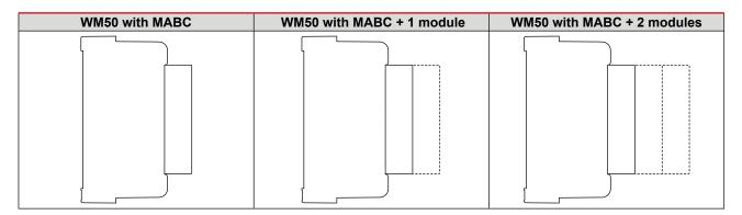
WARNING: maximum 1 module per type. A digital input/output module cannot be connected with an analog input module.
