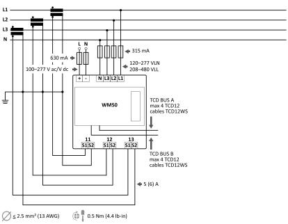
Fig. 1 Three-phase system with neutral (4-wire).
