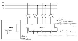
Fig. 13 Two-phase system with neutral (3-wire)
