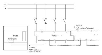
Fig. 12 Single-phase system with neutral (2-wire)
