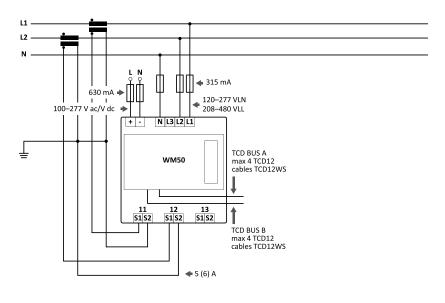
Fig. 2 Two-phase system with neutral (3-wire)
