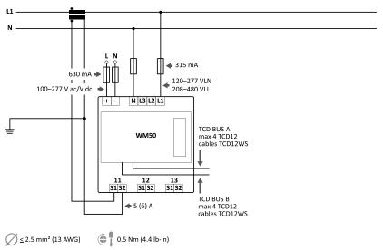
Fig. 3 Single-phase system with neutral (2-wire)
