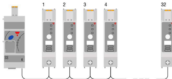
In case of an RG..N replacement, or any changes to the NRG bus chain, the RG..Ns have to be re-addressed. Follow the procedure below to re-address the RG..Ns on the NRG bus chain manually. Alternatively, auto-addressing can be done via an 'Explicit' command (check NRG EtherNet/IP User Manual for further information)
