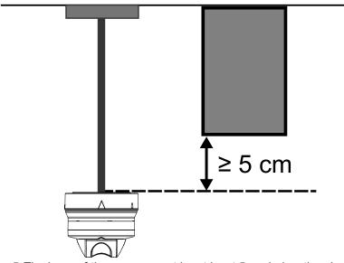
Fig. 5 The base of the sensor must be at least 5 cm below the obstacle
