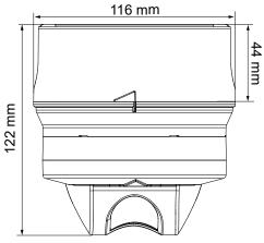
Fig. 2 Ceiling mounting - base B + Sensor
