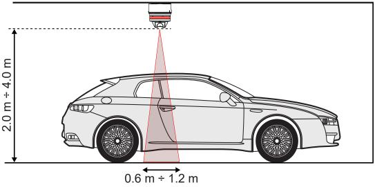
Fig. 3 Sensor height and distance
