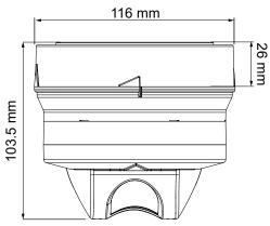
Fig. 1 Rail mounting - base A + Sensor
