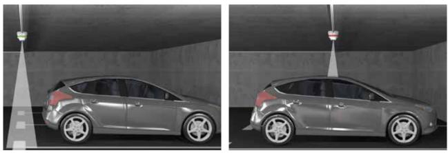
The sensor is wrongly mounted in the lane
