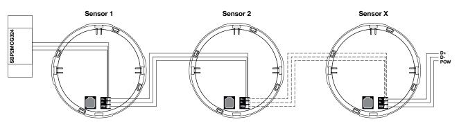
**Note:** The wiring of the sensors must always be made with a 1.5 mm<sup>2</sup> single-core wire, or a stranded wire with ferrules.
