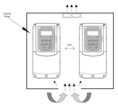
The necessary physical space and cooling should be provided, based on the ambient temperature and the heat loss in the panel.
