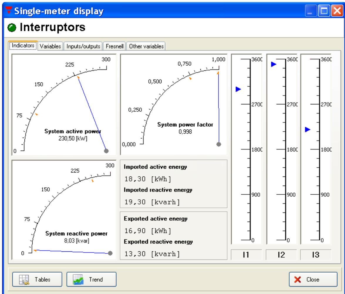
On the top of the page, the name of the instrument and the communication status are shown. The flashing of the green LED indicates that a new reading has been preformed from this meter and that the displayed values have been updated.
