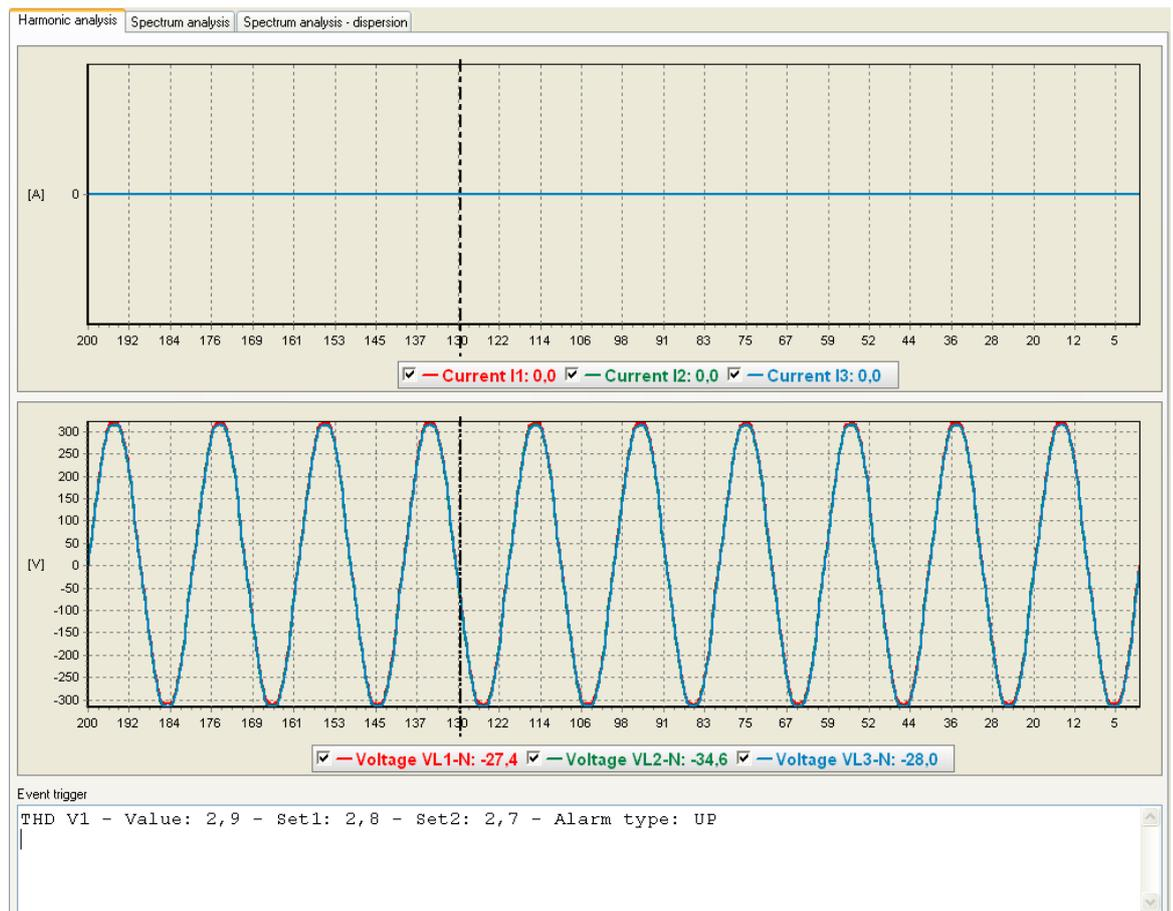
In this section will be showed the time domain analysis for two types of graphs: currents and voltages. All times are expressed in milliseconds, while in the ordinates you can find the Ampere or Volts values.
