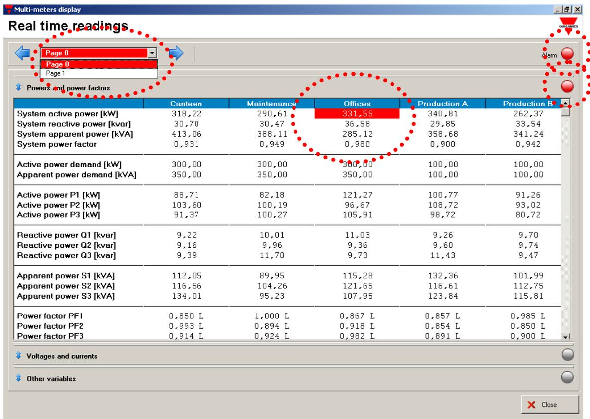
If the alarm condition occurs in an instrument not included in the current page, it is possible to locate the right page looking at the page drop-down menu, where the relevant page is highlighted in red too.
