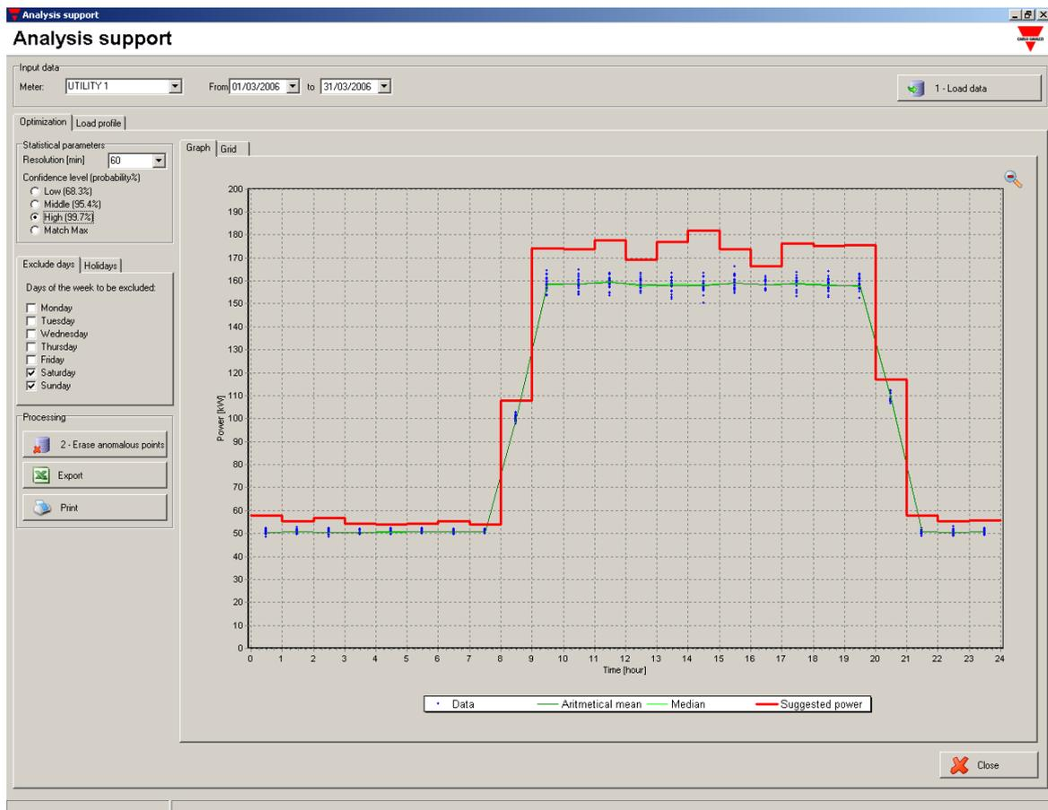
After uploading the data, the statistical parameters are to be properly set. The *Resolution* indicates the duration of the time intervals in which the day is split (from 5 to 60 minutes). The *Confidence level* indicates the probability that the consumptions of the instrument are below the proposed contractual power.
