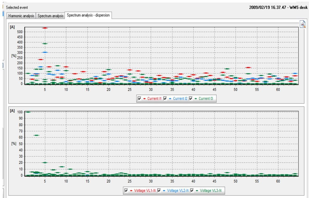
In this page it is showed the spectrum analysis for each current and voltage in the frequency domain. All the harmonics that were downloaded in a file can be displayed in this window in two graphs of dispersion.
