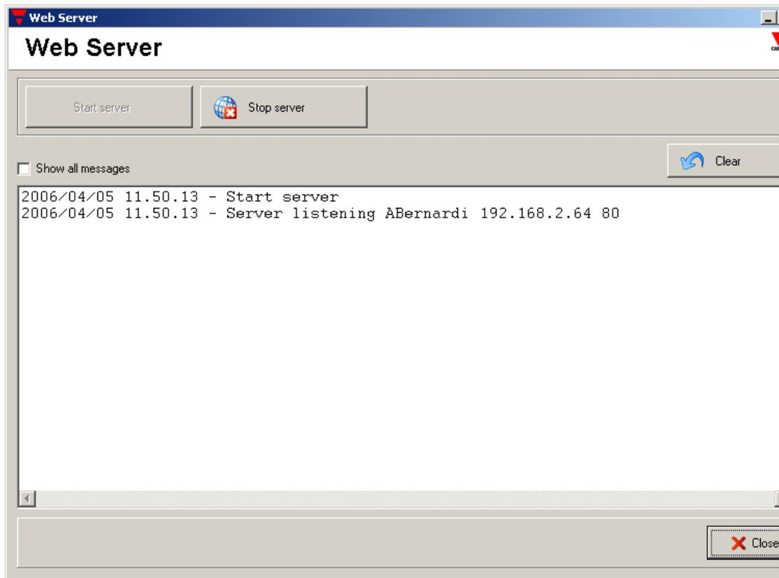
From this window it is possible to activate or deactivate the web server function by means of the relevant buttons. The log of the events relevant to the web server allows the user to be updated on the module status. Only the most important messages are shown, unless the *Show all messages* box is ticked. To clear the log, the relevant button is to be used.
