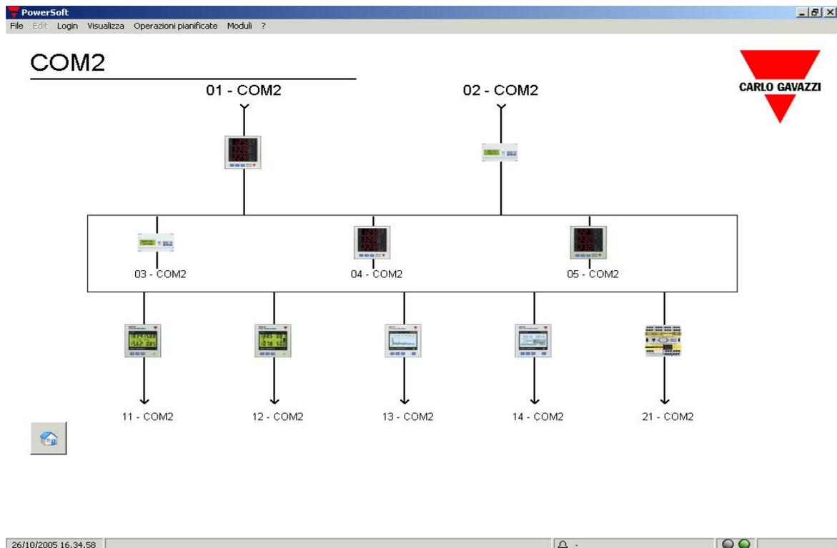
Any alarm status of each instrument is directly available on the synoptic pages: if the instrument is not communicating, a fuchsia square appears around it; if there is a setpoint alarm, the square indication is red.
