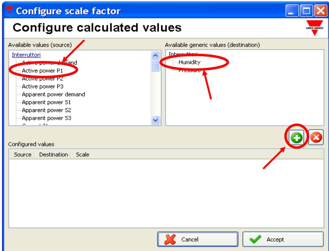
It's possible now to link one of the created variable to one of the available measure by choosing the real measure on the left section of the window and the generic variable that has to be associated at in the right section of the window.
