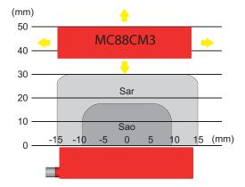
Note: the typical detection characteristic shown may vary from sensor to sensor.
