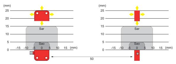
Note: the typical detection characteristic shown may vary from sensor to sensor.
