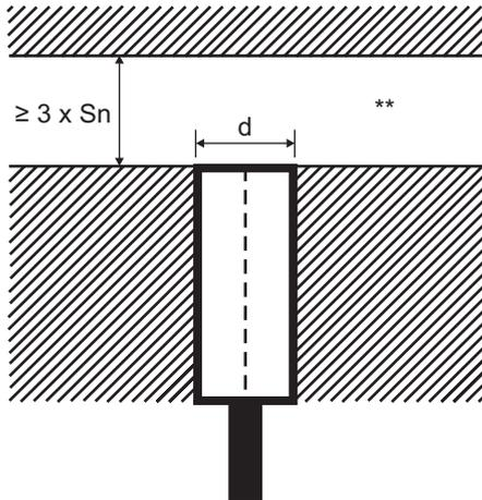
**Fig. 11** Flush sensor, when installed in damping material
