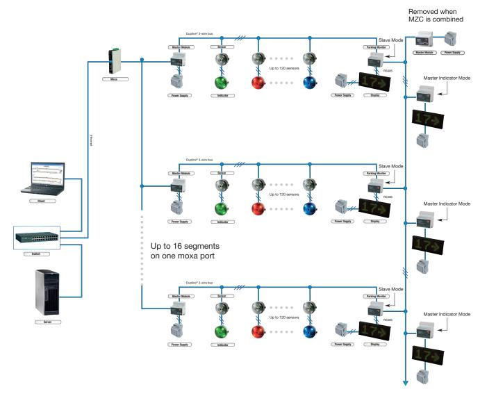
The client (or clients) is also connected to the LAN. The client is the application for the operator of the system, who wants to receive information from the parking facility. The design of the parking facility is done by means of the client, where diagrams, pictures etc. can be uploaded as background for the programming.
