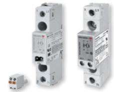
Slim **RGS1** panel mountable solid state relays are only 17.5mm wide. Nominal current ratings include 25, 50, 75 and 90AAC at up to 660VAC. Narrow width and larger output terminals make it ideal compared to standard chassis mount (hockey puck) SSRs.
