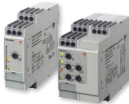
**DUA** AC/DC over voltage monitoring relay and **DUB** TRMS AC/DC over or under voltage monitoring relay. **DUC** features over+under, over+over or under+under voltage monitoring. 11-pin **PUA/PUB/PUC** plug-in types are also available. 500VAC/DC maximum monitoring.
