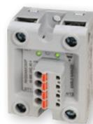
The **RK** is a series of 2-pole SSRs contained in one housing with the possibility to control each pole independently (**RKD2** models) or both poles together (**RK2** models). Ratings are up to 660VAC, 75AAC per pole. Input connectivity options include a 2.54mm male cable connector or a pluggable 5.08mm spring terminal.
