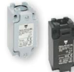
Full-size, standard housing, with one cable/conduit entry. 20 different actuator options. 10 different contact block choices. Positive opening operation, double insulation. Available in metal (IP66) or plastic (IP65) housing. Robust switch in traditional package.
