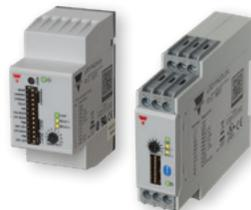
**LDP** and **LDD** Amplifiers single and dual loop types, universal supply voltage 24-240VAC/VDC, plug in and DIN rail mounting. Loop inductance input between 20uH and 1000uH, adjustable sensitivity, 2 SPDT relay outputs. Advanced diagnostics, automatic sensitivity and frequency.
