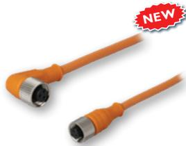
IP67 PVC cordsets, available with straight or right angle M12 connector. 3 pin/wire connection for AC/DC sensors. Cable lengths in 2m and 5m, with other lengths available upon request.
