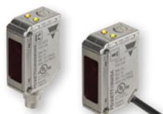
Stainless steel sensors with IP69K ratings, NEMA rated and ECOLAB approved. Rugged design fit for harsh environments, high-pressure washing, abrasive disinfectants and cleaning agents. Available in wide angle diffuse (200mm) and through beam (15m). Background suppression, diffuse, retro-reflective and polarized options available in IO-Link (see page 11).
