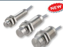
M12, M18, M30 inductive sensors with full stainless steel housing. Easy configuration and advanced monitoring such as low margin alarm, proximity alarm, or activation level via IO-Link. Suitable for harsh environments with IP69K and -40 to 85°C and up to 100°C for 15 minutes. M12 flush (4mm) or non-flush (8mm), M18 flush (8mm) or non-flush (14mm), M30 flush (15mm) or non-flush (22mm) sensing.
