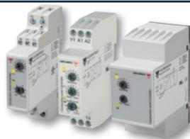
Dual-point level controller for conductive liquids, which can control up to two levels of filling or emptying. Adjustment sensitivity from 250 $\Omega$  to 500K $\Omega$ . DIN rail mount (**CLD2**) or 11-pin plug-in (**CLP2**). Supply voltage of 24VAC/DC, 115VAC or 230VAC. **CLD2EB1BU** is 240VAC/DC. Up to two 8A outputs and diagnostic LEDs.
