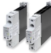
Mini size **RGC1** solid state relays and contactors with integrated heat sink maximize panel space. Up to 25AAC/3Hp in 17.5mm width and up to 30AAC / 5Hp in 22.5mm width. Up to 1,800 A2s I2t and 1,200 Vp blocking voltage. Nominal rating at 40°C. IP20 and MOV protection standard.
