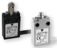
Miniature limit switch with 20mm mounting hole spacing. Pre-wired with 1m (3.3 ft.) of cable, right exit. 15 different actuator options. 2 different contact block choices. Double insulation, positive opening operation. Available in metal or plastic housing. Fully potted, IP67 rated.
