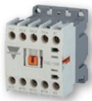
Electromechanical 3-phase switching. AC3 480VAC rating 6, 9 and 12AAC. cUL ratings up to 7.5Hp. One auxiliary contact. Full arrangement of AC and DC coils and accessories. Connection choices of screw, cage clamp, fast-on and pin terminals.
