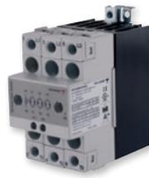
Two-pole, three-phase, zero-switching, **RGC2A** solid state contactors are ideal for applications where frequent switching is required. Maximum rating per pole is 75AAC/25Hp at 40°C, 660VAC. MOV and snubber protection are standard.
