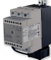
Three-pole, three-phase, zero-switching, **RGC3A** solid state contactors can be used in 3-phase applications where all poles must open. Max. rating per pole is 65AAC/25Hp at 40°C, 660VAC. MOV and snubbers are standard.
