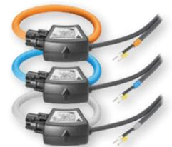
**ROG4** series Rogowski coil current sensors are flexible, easy to install, and highly accurate. For measuring currents up to 4000A, with output of 100-120mV. External coil diameters range from 90 to 290mm. Accuracy to +/- 1%.
