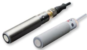
Multi-function M18 diffuse ultrasonic sensor in IP67 PBT plastic or stainless steel housing. Sensing distance up to 2.2m. Two transistor outputs, or one analog and transistor output. Standard switching, adjustable hysteresis or window modes via a simple pushbutton set-up. 2m cable or M12 plug connection.
