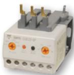
Electronic overloads use solid state technology to detect overload and phase loss, as well as phase reversal and unbalance. Wide overload range and user selectable trip class. Three frame sizes, protecting motors from 0.3-85AAC. Direct, separate and through-hole mounting styles.
