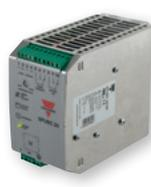
Modular single phase power supplies feature a low profile depth of 2.2" (58mm). Output power levels consist of 15, 24, 36, 54, 60, 90, and 100W in voltages of 12 and 24 VDC. Models <100W are UL62368 Low Power Source (LPS) compliant.
