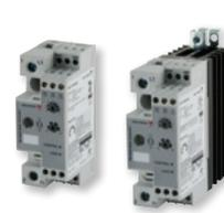
Analog switching **RGS1P** SCR with integrated heat sink is a single pole device that provides proportional output control. This microprocessor controlled device offers the flexibility of five switching modes in one flexible package: Maximum current range is 63AAC, controlled by 4-20mA, 0-5, 1-5 or 0-10VDC.
