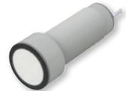
Multi-function M30 diffuse ultrasonic sensor in IP67 PBT plastic housing, with a Ø40 head that protrudes 20mm. Sensing distance up to 6m. Two transistor outputs, or one analog and transistor output. Standard switching, adjustable hysteresis or window modes via a simple pushbutton set-up. 2m cable or M12 plug connection.
