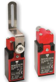
Safety switch used to monitor swinging guard doors and restrict machine operation when safety doors are not properly closed. Double insulation, positive opening operation. Switch mounts on top of machine, and pin is inserted into the door hinge or lever, typically secured to top of door. 2 different housing size options.
