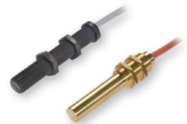
M16 cylindrical proximity magnetic sensors in plastic (FSB) or brass (FSM) housing. PVC or silicon cable. Change over output function. Operating distance up to 8mm depending on the magnet. High temperature sensor.
