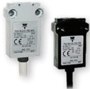
Miniature limit switch with 25mm mounting hole spacing. Pre-wired with 1m (3.3 ft.) of cable. 15 different actuator options. 2 different contact block choices. Double insulation, positive opening operation. Available in metal or plastic housing. Fully potted with IP67 rating.
