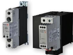
Single phase **RGC1** solid state contactors can be used to control resistive loads as well as be part of AC induction motors starter. UL approved Hp ratings range from 1/3Hp (AC53α: 5A) at 115VAC to 15Hp (AC53α: 20A) at 660VAC. Robust construction of the **RGC1** family allows for up to 30 starts per hour.
