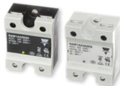
The single phase, chassis mount relay can be used for resistive and inductive loads. **RAM1A** zero switching type and **RAM1B** instant-on type, are available in 25, 50, 75, 100, and 125AAC outputs, for up to 690VAC. The built-in snubber secures transient protection. **RAM1A..G** is Glow wire Certified according to UL60335-1 and offers integrated overvoltage protection.
