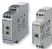
Multi-voltage delay on release (**DBA**) and true delay on release (**DBB**) series are available with up to seven time ranges covering 0.1 second to 100 hours. SPDT or DPDT relay output. Each features simple setup and clearly marked front knobs. 11-pin plug-in versions are also offered (**PBA/PBB**).
