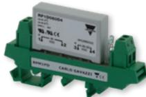
**RP1D...M1/2** is a DC PCB SSRs that is factory mounted on a DIN rail adapter. The device is rated either 1, 4 or 8ADC at up to 60 (M1 suffix) or 350VDC (M2 suffix). The RP1D relay is ideal for applications where there is a need for fast switching of small DC loads.
