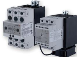
These two and three pole products are solid state alternatives to electromechanical contactors. **RGC2A** or **RGC3A** offer maximum motor rating of 28AAC / 25HP at 660VAC and 40°C. MOV and snubber protection are standard. Models with system monitoring, over-temperature alarm and auxiliary output are available.
