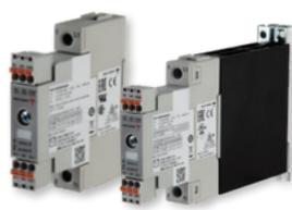
The **RG1..M** solid state devices incorporate monitoring functions for detection of mains and load loss, SSR open and short circuits and internal faults. The RGS1A..M is rated up to 90AAC with proper heat sink, while the RGC1..M is rated up to 65A. Line voltage rating is up to 660VAC.
