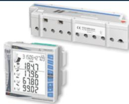
Multichannel power analyzer. Using the **TCD12** split-core current sensors, the **WM50** can monitor any combination of single, two and three-phase loads for a maximum of 96 channels. Optional modules: Modbus-RTU or TCP/IP communication, I/O module or analog and temperature probe input module. Meter is rated up to 550VAC.
