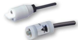
Conductive level sensing probes for liquid level detection. Hanging probe for single level point detection in swimming pools. 5m Neoprene cable connections. The **A94** has two probes in one part, separated by an insulating barrier constructed of the polyester housing material. Detection functions determined by the amplifier used.
