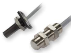
M10 cylindrical proximity magnetic sensors in nickel plated brass housing. PVC cable with NO, and NC output function. Operating distance up to 23mm.
