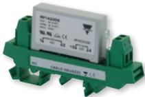
**RP1A** or **RP1B** are solid state relays for printed circuit board mounting, but when ordered with M1 (230VAC) or M2 (480VAC) suffix, they leave factory attached to a DIN rail adapter. Voltage rating includes 230VAC (12.5mm wide) and 480VAC (25mm wide), current rating up to 5.5AAC.
