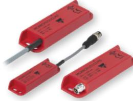
Encoded safety magnetic sensors, IP67 PBT housing (88 x 25 x 13mm) rated from -25 to 80°C (-13 to 176°F). Left or right exit, 2m cable, M8 or Pigtail M12, with or without LED indicator. Offered with 2 or 3 outputs (2NO, 1NO and 1NC, 2NO&1NC). Safe switch on distances up to 18mm and a safe switch-off distances of up to 30mm using the **MC88CM** coded actuators.
