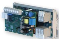
The **HDMS** is a soft starter for single phase scroll compressors, hydraulic and submersible pumps up to 253VAC and 37AAC. Through an innovative control strategy, Capacitor Start-Capacitor Run motors can now be started without a start capacitor. Modbus RTU, NFC and class 10 overload are standard.
