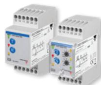
Earth leakage monitoring relay, used with core balance current transformer (**CTG**) and circuit breakers to provide protection against fault currents and to reduce fire hazards. **DEA71** has fixed settings for fast installation, and **DEB71** has adjustable sensing ranges and time delay to customize for any application.
