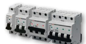
UL 1077 supplementary protectors offer overcurrent protection for specific applications where branch circuit protection is already provided by another device or is not required. Product is available in 1, 2, and 3-pole variations, ranging from 1 to 63Amps and has a short circuit rating of 5kA.
