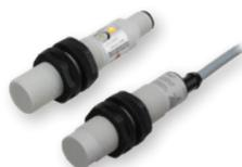
Capacitive proximity sensors, TRIPLESIELD™ technology. AC, AC/DC 2 wire or DC 4 wire. High immunity to EMI, dust and humidity compensation. Flush, non-Flush, IP67, IP69K. Thermoplastic. Sensing ranges up to 12mm. Teach-in DC versions available. NPN, PNP (or auto-detect), SCR, NO & NC output. Dust or temperature alarm DC versions. 2m cable or M12 plug.
