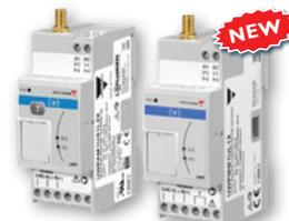
**UWPA** is an endpoint adapter that provides LoRa® or LoRaWAN® communication to an RS485 Carlo Gavazzi meter. **UWPM** is a master concentrator that permits **UWP 4.0** to gather data from multiple **UWPA**. Up to 10km range is possible, with embedded end-to-end AES 128 encryption. Low operating costs, with no SIM cards or fees.
