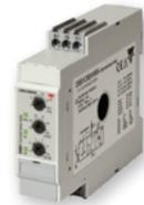
The **DIB Series** TRMS AC over or under current monitoring relay with a built-in current transformer that measures from 2A to 100A AC. Through-hole size of 12mm.
