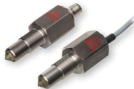
High end optical level sensors with modulated infrared light with built-in amplifier. 4 wire, DC voltage supply, NPN, PNP, NO and NC output. Stainless steel or nickel-plated brass housings, with glass or polysulfone tip resistant to most acids and bases. 2m oil resistant cable or M12 connector.
