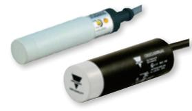
ATEX approved Capacitive AC or DC proximity sensors, Ø18 & Ø32 mm (TRIPLESIELD™). IP67, sensing distances up to 12mm (Ø18) and up to 20mm (Ø32) non-flush mount. NO or NC with ON or OFF delay output (AC models), relay, SCR, NPN or PNP with NO or NC output (DC models). Ideal for detecting grain or solids in tanks, silos or containers in ATEX Zones 20 or 22.
