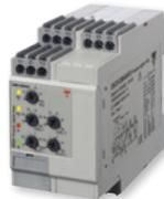
TRMS AC/DC over+under, over+over or under+under current and voltage monitoring relays. **DIC01** can also perform +/- DC measurement. 11-pin **PIC** plug-in types are also available. 10V maximum monitoring; up to 500AAC (1 or 3-phase) with an **MI** or **MP** CT.
