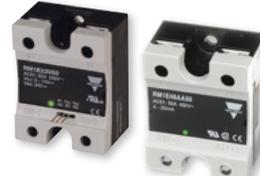
The analog switching relay works in accordance with the phase angle control principle, where the switching point and voltage at the output varies proportionally to the proportional input which can be 4-20mA or 0-10VDC. **RM1E** offers output ratings of 25, 50, 75 and 100AAC at up to 660VAC.
