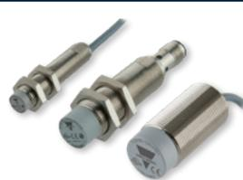
M12, M18, M30 inductive sensors in short or long metal housing. Configurable via IO-Link with application functions of frequency monitoring and RPM counter. M12 flush (4mm) or non-flush (8mm), M18 flush (8mm) or non-flush (14mm), M30 flush (15mm) or non-flush (22mm) sensing.
