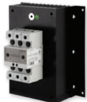
**RGC3A..48** is a three-pole, three-phase variant of the RGC3A, where a conventional, DIN-rail mountable heat sink is replaced with one that can be panel or thru-wall mounted. Amperage rating of 48AAC/25Hp at 40°C per phase is achieved without the use of a cooling fan.
