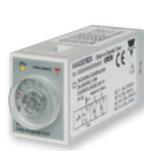
This popular miniature housing provides multifunction and multi-voltage supply with just two models, a DPDT (**HAA08**) and 4PDT (**HAA14**). Each features delay on operate, symmetrical recycler "ON" first, symmetrical recycler "OFF" first and Interval timing functions.
