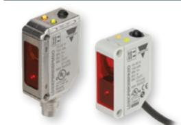
Miniature size IP67 plastic housing or IP69K ECOLAB certified stainless steel housing with red or infrared light. Available in diffuse reflective (1m), polarized retro-reflective (6m), and background suppression (200mm, 250mm, 350mm). Applications functions included: pattern recognition, speed & length, divider, object & gap monitoring.
