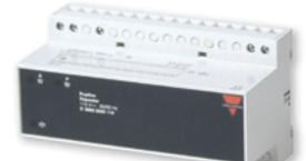
The Dupline repeater functions to regenerate the Dupline carrier signal in order to extend the bus up to another 10Km (6.2 miles). This category includes optical repeaters for sending the signals over fiber optic transmission cables.
