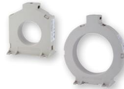
**CTG** core balance transformer used with **DEA71** and **DEB71** to detect residual current on monitored line. Provides output when a current imbalance is detected. 6 models with through hole sizes from 35mm to 210mm.
