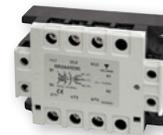
The **RR2A** is solid state reversing relay for 3-phase induction motors. LED indication for "forward" and "reverse" mode indication. Motor rating: three phase up to 7.5 Hp. The output is protected from excessive voltage fluctuations (transients) by built-in varistors.
