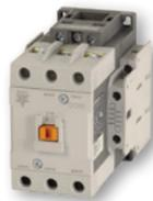
Rugged 3 or 4-pole contactors with AC3 480VAC ratings of 9-100AAC, cUL ratings of 5-75Hp. Full range of AC or DC coils. Screw and lug terminals. One or two sets of auxiliary contacts. Accessories include overloads, reversing kits, extra auxiliary contacts and surge suppression units.
