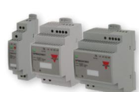
Single phase DIN-rail mount power supplies offer high performance within an extremely compact footprint. Power ratings from 75 to 480 W with 12, 24 & 48 VDC output. Efficiency rating of up to 94% at 230 VAC. Features such as DC OK output relay (for **SPDE..R** models) and built-in protection functions ensure a high degree of reliability.
