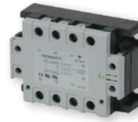
This heat sink mountable 3-phase zero switching **RZ3A** SSR is designed to switch resistive and inductive loads up to 75 and 20AAC respectively, at up to 660VAC. Built-in varistors provide transient protection for heavy industrial applications. Optional over-temperature protection is also offered.
