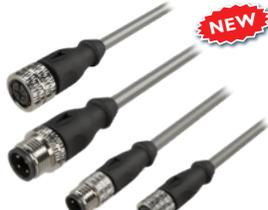
IP68 PVC double-ended cordsets available straight or right angle, M12 or M8 connectors, 3 or 4 pin/wire connection for DC sensors. Cable lengths in 2m and 5m, with other lengths available upon request.
