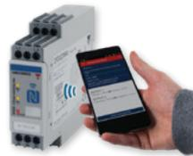
3-phase voltage and frequency monitoring relay provides protection against phase reversal/loss and if the phase asymmetry, voltage or frequency are not within the user-configured settings. The **DPD** settings can be modified through a smartphone/tablet or via a USB NFC Reader/Writer. 552VAC maximum monitoring.
