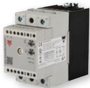
The **RGTS** is a full solid-state, compact and easy to use soft starter for single phase two wire AC induction motors. Motor ramp-up time and initial torque can be adjusted through the built-in potentiometers. Three amperage ratings are available; 12, 16 and 25AAC, while the operational voltage range is 100-240VAC.
