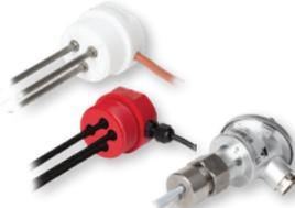
Level sensing probes to control filling and emptying of conductive liquids. Use with **CLD/P** controllers below. Includes up to four insulated or non-insulated electrodes 1 meter long, cut to length to suit the application. Housings available in nylon (**VN**), PVC (**VPC**), polypropylene (**VPP**), food grade stainless steel (**VS**), and Teflon (**VT**).
