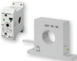
The **E83 Series** compact AC current metering transducer with 7 selectable primary ranges up to 50AAC and a 12mm through hole. Also offered in a cabled version, the **A82 Series** comes in a 25, 50, 100, 250 and 500AAC primary range with a 0-20mA, 4-20mA or 0-10VDC output and 27mm through hole.
