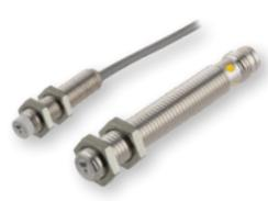
Inductive proximity sensors in M8, M12, M18 and M30 stainless steel & nickel plated brass IP67 housings. Sensing ranges up to 4mm (M8, M12), 8mm (M18) and 15mm (M30). NAMUR, 2 wire DC and 3 wire DC options. Flush or non-flush mounting. M8, M12 or 2m cable connection.
