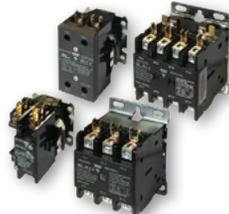
Cost-effective range of contactors offered in single, single+shunt, two and four pole normally open contact arrangements for 25-40AAC maximum AC3 ratings with screw or lug load terminals standard and in three pole from 25-90AAC with lug load terminals standard. Multiple 0.25" fast-ons are also standard for control and load terminals.
