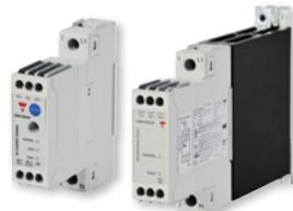
This **RG** design is capable of load switching as well as detecting of full or partial load failures, open or short SSR circuit, and SSR over temperature. Product is available in versions without heat sink (**RGS1S**) or with heat sink (**RGC1S**). Available current range is up to 85AAC at 40°C.
