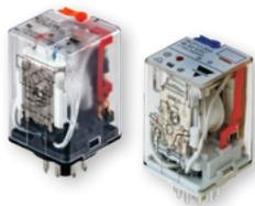
2 and 3 pole relays for a wide range of industrial applications. Available in 8 or 11 pin versions from 6VDC-110VDC and 6VAC-230VAC. Up to 10AAC output contacts. Pair with **ZDP** sockets.
