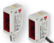
Compact size through-beam sensors in a reinforced plastic housing. High accuracy in a small package. Top or back potentiometer adjustment. 15m sensing distance. Remote teach, mute function or dust alarm options available. Background suppression, diffuse, retro-reflective and polarized options available in IO-Link (see page 11).
