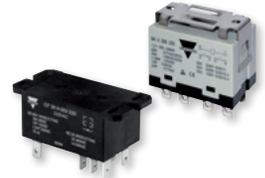
High power relay, in a sealed design, ideal for vending machines, copiers, compressors and control equipment. Switching capacity up to 30AAC. Reinforced insulation 4 kV / 8 mm (0.31").
