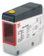
Full size range of AC/DC or DC-sensors in a reinforced plastic housing. Diffuse (0.8m), retro reflective (10m), polarized retro reflective (12m) and through beam (20m). Mute input to verify sensing function. Ideal for industrial and door applications. UL325 approval.
