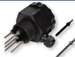
Modular level sensing probes to control filling and emptying of conductive liquids. Use with **CLD/P** controllers below. Up to five **CLE** insulated or non-insulated electrodes can be used. Probes are 1m long and add up to virtually any length as required by the application. Kynar (PVDF) and polyolefine (FR) electrode insulation available.
