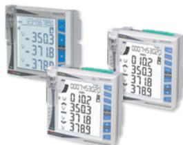
Modular power analyzers for 3-phase systems up to 690VAC, with simplified user interface and LCD data display. Options include optical port, Modbus-RTU, BACnet-IP, or Profibus-DP comms. **WM20** supports 2 outputs. **WM30** supports 4 outputs and is Go Solar California eligible. **WM40** supports 6 inputs (for utility metering) and 8 outputs, with built-in datalogger.
