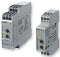
Our multi-voltage delay on operate timer with seven time ranges covering 0.1 second to 100 hours. SPDT or DPDT relay output. Clearly marked front knobs allow simple setup. 11-pin plug-in version is also offered (**PAA**).
