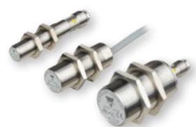
**ICS-E1** Series high performance for harsh environments. M12, M18 and M30 stainless steel housings. IP69K rated, -40 to 85°C (-40 to 185°F) operating temp. 3 wire, 8-60VDC. Flush or non-flush, up to 22mm sensing distance. High EMC immunity, load dump protection. Connection choice of 2m PUR cable or M12 plug. E1 approval for mobile equipment.
