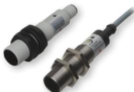
Supply voltage 20 to 250VAC. Nickel plated brass or thermoplastic housings, IP67. Diffuse (400mm), polarized (2m), retro-reflective (3m) with immunity to reflecting surfaces. 2-wire, NO or NC SCR output type. 2m PVC cable or M12 plug.
