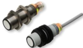
Short bodied multi-function multi-function M18 diffuse ultrasonic sensor in IP67 PBT plastic or stainless steel housing. Sensing distance up to 2.2m. Two transistor outputs, or one analog and transistor output. Standard switching, adjustable hysteresis or window modes via a simple pushbutton set-up. 2m cable or M12 plug connection.
