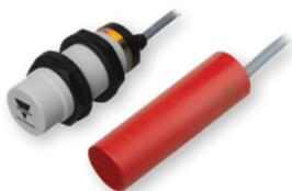
Capacitive level sensor for solid, fluid or granulated substances, in M30 PBTP threaded housing or smooth Ø32 thermoplastic housing (for PG36 screw gland). 21-265VAC/DC supply and 2A SPDT output. Adjustable sensing distance up to 12mm. Versions with adjustable (ON or OFF) time delay.
