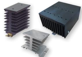
**RHS** Heat sinks are a necessary accessory for any chassis mount relay where more than 5 amps are being switched. Available for DIN rail, panel and through-the-wall mounting of one to multiple SSRs, the product offering dissipates from 4.0 to 0.12°C/W. Optional cooling fans are also offered.
