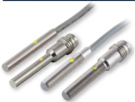
Miniature inductive sensors in stainless steel housings. Smooth Ø4mm (IBS) or threaded M5 (ICS) barrels are IP67 and -25 to 70°C / -13 to 158°F rated. Flush mount sensing up to 1.3mm, with detection speeds up to 6Khz.
