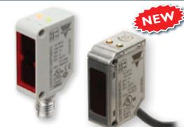
Laser time of flight measurement allows reliable and accurate detection even at longer distances. IP67 plastic housing or IP69K ECOLAB certified stainless steel housing for washdown environments. Diffuse (1m), retro-reflective (6m), and background suppression (200mm, 250mm, 350mm). Applications functions include pattern recognition, speed length, divider, object & gap monitoring.
