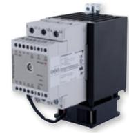
The **RGC2/3P** solid state controllers, provide proportional output control. This microprocessor controlled device offers several switching modes such as phase angle, full distributed cycle or soft start. Maximum current range is up to 75AAC (**RGC2P**) and 65AAC (**RGC3P**), controlled by several types of analog input signals.
