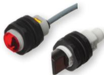
M18 family of cost-effective general purpose DC 4-wire sensors in IP69K plastic housings (axial and radial type). Background suppression (200mm), diffuse (1m), diffuse wide angle (0.4m), polarized (5m), retro-reflective (6.5m), through-beam (20m). 2m PVC cable or M12 plug. Sensors are ECOLAB approved.
