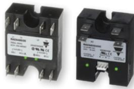
2-pole SSR minimizes the space requirements without compromising performance. Two SSRs are built into a single **RA2A** 'hockey puck' SSR. Relay is rated up to 40AAC per pole, up to 660VAC. 0.25" fast-on terminals are utilized on output terminals for quick wiring. Choice of fast-on or pin-header for input voltage.
