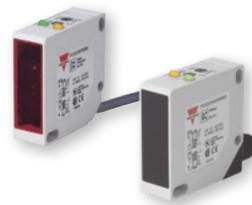
Compact size of full range AC/DC or DC 4 wire sensors in a reinforced plastic housing. Diffuse reflective (1m), background suppression (500mm), retro reflective (10m), polarized (6m) and through beam (20m). NO and NC, NPN, PNP or Relay output. The long sensing range and sensitivity adjustment make for a very flexible sensor. 2m cable or M12 swivel connector
