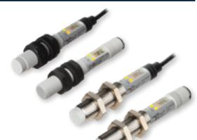
M12, M18, M30 capacitive sensors in plastic or stainless steel housing. Configurable via IO-Link: output type, time delay, logic gates, output inverter, dust alarms, external teach and diagnostics. M12 flush (4mm) or non-flush (8mm), M18 flush (8mm) or non-flush (12mm), M30 flush (16mm) or non-flush (25mm) sensing.
