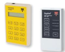
The hand-held configuration unit for DuplineSafe quickly connects to, and programs the sensors and monitors. It features an LCD display and 12-key tactile keyboard, powered by a standard 9VDC battery. The more compact programming and test unit is for Dupline Industrial.
