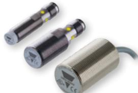
**ICB** Series in M12, M18 and M30 nickel plated brass IP67 housings. Sensing range up to 10mm (M12), 20mm (M18) and 40mm (M30). 3 wire DC output. Quasi-flush or non-flush mounting. Connection choice of 2m cable or M12 plug. IO-link versions of these sensors are shown on page 11.
