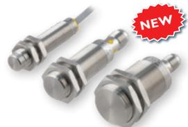
**ICF** Series full stainless steel housing in M12, M18 and M30. Metal face resistant up to 260 bar pressure (M12). Extended sensing ranges up to 22mm (M30), 14mm (M18), 8mm (M12). IP69K, ECOLAB certified, rated from -40 to 85°C (-40 to 185°F). 3 wire DC. Flush or non-flush mounting. IO-link communications on board, more info on page 11.
