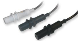
Capacitive proximity sensors with TRIPLESIELD™ technology. Adjustable sensing distance of 3-8mm (flush) or 3-12mm (non-flush). M18 cylindrical in polypropylene (black), PVC or Teflon housings with 2m cable. Ideal for use in level applications in chemical, semiconductor and food & beverage industries.
