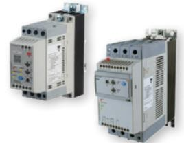
The **RSGD** is an extremely compact and easy to use 3-phase soft starter for AC induction motors rated up to 100Arms. The starting parameters can be easily setup through 3 selector switches. The integrated motor overload protection (Class 10) and Modbus communication on larger frame models, result in a higher installation flexibility.
