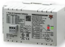
Compact single phase scroll compressor soft starter with integrated start capacitor. **RSBS** is available in standard 25A and High Pressure 32A sizes. High Pressure version provides a dynamic current limiting that ensures compressor starting even at higher starting pressures with maximum current limit of 80AAC.
