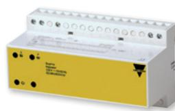
Passive gateway with safety mapping is DIN-rail mounted and reads and controls up to 128 inputs and outputs through Profibus-DP. Also offered is an isolated DuplineSafe repeater, for extending the transmission distance. These can be cascaded.
