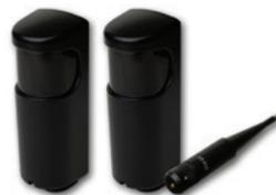
UL325 sensors for door or gate widths up to 60m. 24VAC/DC supply with a SPDT relay output. Adj. lenses in the horizontal (200°) and vertical planes (30°). Rugged vandal resistant, aluminum and polycarbonate housing. Optional **ADP Series** green laser alignment tool. UL325 approval.
