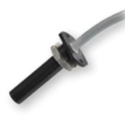
Cylindrical proximity magnetic sensor in Ø 13.5 plastic housing. PVC cable with NO, NC, and change over output function. Operating distance up to 12mm.
