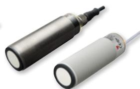
Multi-function M30 diffuse ultrasonic sensor in IP67 PBT plastic or stainless steel housing. Sensing distance up to 3.5m. Two transistor outputs, or one analog and transistor output. Standard switching, adjustable hysteresis or window modes via a simple pushbutton set-up. 2m cable or M12 plug connection.
