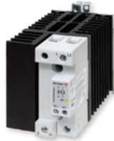
Power line of the **RGC1** with maximum output rating of 85AAC/15Hp at 40°C. 65AAC/15Hp version uses natural air convection cooling, while the 85AAC/15Hp version uses a built-in fan to achieve its high rating. MOV protection is standard. 100KAAC SCCR UL508 rating.
