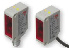
High sensing performance using PointSpot light source, which eliminates any halo effect. Background suppression (250mm) and polarized retroreflective (5m). 4 wire DC. Potentiometer adjustment. NPN or PNP, with NO and NC output function. IP67 housing. PointSpot sensors with IO-Link are also available, (see page 11).
