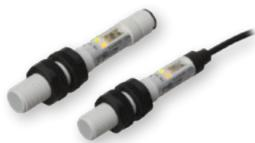
Capacitive proximity sensors, TRIPLESIELD™ technology, high immunity to EMI, humidity compensation. Thermoplastic housing, IP67 rated, -20 to +85°C (-4 to +185°F) operating temperature. Sensing ranges up to 8mm. Teach in button or wire. 4 wire DC, NPN or PNP auto-detection with programmable NO or NC output and alarm output. 2m cable or M12 plug.
