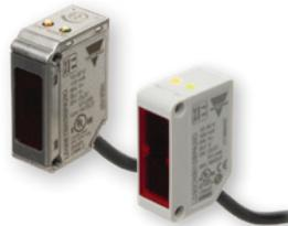
Laser time of flight measurement allows reliable and accurate detection even at longer distances. IP67 plastic housing or IP69K ECOLAB certified stainless steel housing for washdown environments. Diffuse (1m), retro-reflective (6m), and background suppression (200mm, 250mm, 350mm). IO-Link functionality (see page 11).
