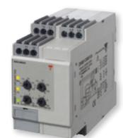
Over or under Cos  $\Phi$  monitoring relay (**DWA**) and TRMS AC active power and power factor monitoring relay (**DWB**) for balanced 3-phase system. 11-pin **PWA** plug-in types are also available. 480VAC max. monitoring, maximum current is determined by the primary of the **MI**, **MP** or 5A secondary CT.
