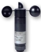
Cup anemometer with optoelectronic detection for measuring air speed. Built-in heater and dust sealing. Inputs and outputs protected against reverse polarity and transients.
