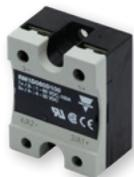
The **RM1D** SSRs are used in fast switching applications of small DC loads with high input/output isolation of 3,750Vrms. The DC output switches ON and OFF in accordance with the applied DC control voltage. Outputs of up to 100A at a maximum of 60VDC, up to 50A at a maximum of 200VDC, and up to 10A at a maximum of 500VDC.
