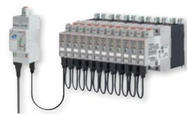
The **NRG** is a system consisting of a master controller and up to 32 slave **RG..N** solid state relays and contactors. The **NRG** system offers control and monitoring via Modbus, ProfiNet, EthernetIP, EtherCAT, and Modbus TCP. The **RGS1A..N** is rated up to 90AAC with proper heat sink, while the **RGC1..N** is rated up to 65AAC with integrated heat sink.
