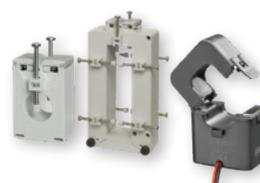
Full range of current transformers and sensors. DIN-rail, cable or bus-bar mounting options include solid core **CTDX** or split core **CTDS** series, rated up to 3200A primary with 1A or 5A secondary. Miniature cable mount split core options include **CTA** series with input up to 600A and 5A secondary, and **CTV** series with input up to 800A and 333 mV output.
