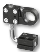
Universal mounting bracket for all cylindrical sensors with  $\varnothing 4$  to  $\varnothing 30$  mm. The mounting adaptor is supplied complete with 2 mounting heads ( $\varnothing 18$  and  $\varnothing 30$  mm) and 5 adaptor bushings ( $\varnothing 4$ ,  $\varnothing 5$ ,  $\varnothing 8$ ,  $\varnothing 12$  and  $\varnothing 14$  mm).
