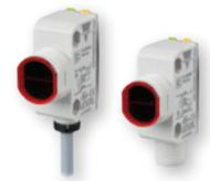
Small sensors ECOLAB approved in versatile IP69K housings provide for side mounting with screws, or front mounting with the 18mm threaded barrel. Potentiometer adjustment, available in diffuse (1m), background suppression (200mm), polarized (5m), retroreflective (6.5m), through beam (20m) sensing functions. 2m PVC cable or M12 plug.
