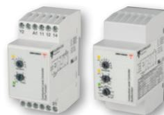
Multi-point level controller for conductive liquids, which can control up to four levels of filling or emptying. Adjustment sensitivity from 250 $\Omega$  to 500K $\Omega$ . DIN rail mount (**CLD4**) or 11-pin plug-in (**CLP4**). Supply voltage of 24VAC/DC, 115VAC or 230VAC. Two 8A outputs and diagnostic LEDs.
