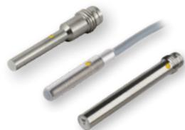
Miniature inductive proximity sensors with sensing ranges up to 1.3mm. 3 wire DC. M5 threaded, 4mm and 6.5mm smooth barrel. Stainless steel, IP67 housing. Flush or non-flush mounting. M8 or 2m cable connection. 6khz speed. IO-link versions of these sensors are shown on page 11.
