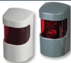
Versatile polarized retroreflective sensor for automatic door systems. IP66 plastic or metal alloy housing. Detects in one of three directions by adjusting the sensing angle within the housing. 24VAC/DC supply, Relay output, with up to 12m range. UL325 approval.
