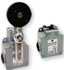
Large standard housing, with three cable/conduit entries. 20 different actuator options. 10 different contact block choices. Positive opening operation. Available in metal (IP66) housing. Robust switch in large package.
