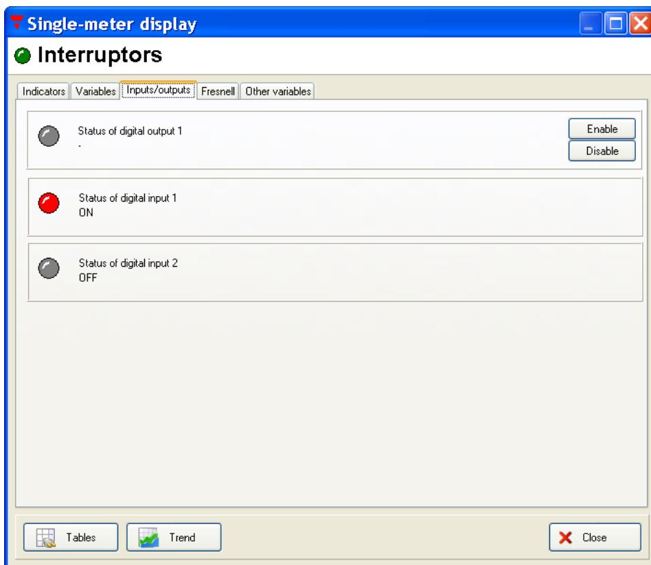
The status is indicated by means of both an ON/OFF text and a status LED (respectively red/grey). If the inputs/output are not configured, they are shown in this section as not available.
