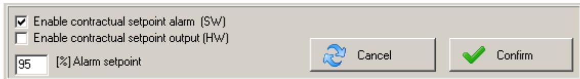
The alarm can be software only or software and hardware as per the other alarms.
