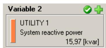
In the legend the name of the variable, the relevant instrument, and the value (with the engineering unit) which is pointed by the mouse cursor in
