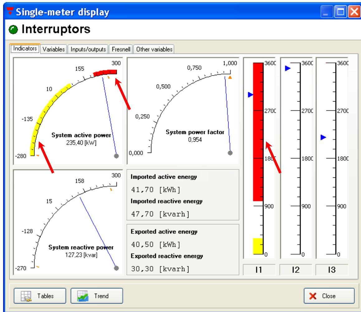
In the above picture, the red arrows show the setpoint values assigned to the variables (system active power and current phase 1 in the example). Two setpoints are available for each variable: an upper setpoint (red band, “up” type alarm) and lower setpoint (yellow band, “down” type alarm). The minimum and maximum values reached by the variable from the previous recording (variable data log on the hard disk) are shown by means of two amber indicators, close to the scale.
