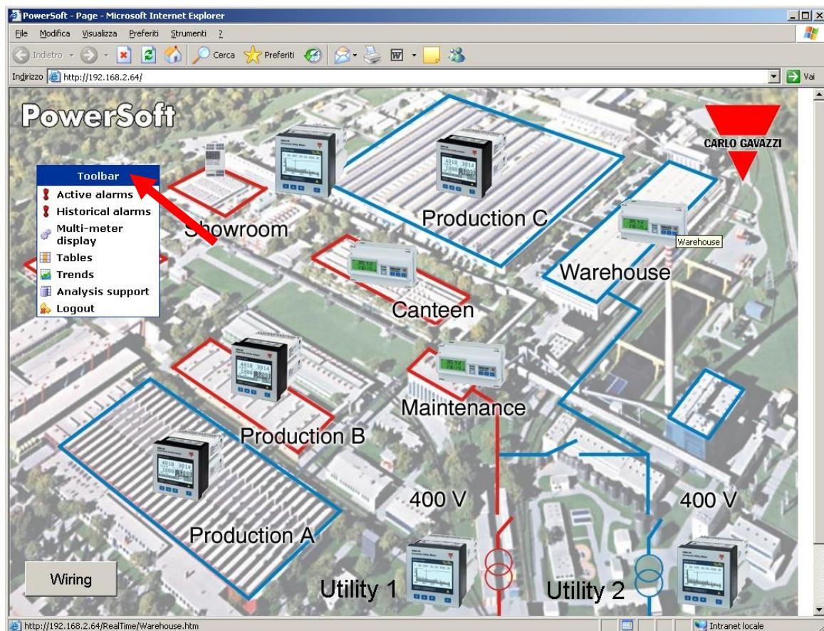
The toolbar allows activating all the functions of the installed modules. Clicking any available entry on the toolbar, a new Explorer window, where the parameters necessary to the execution of the required report are to be entered, is opened.
