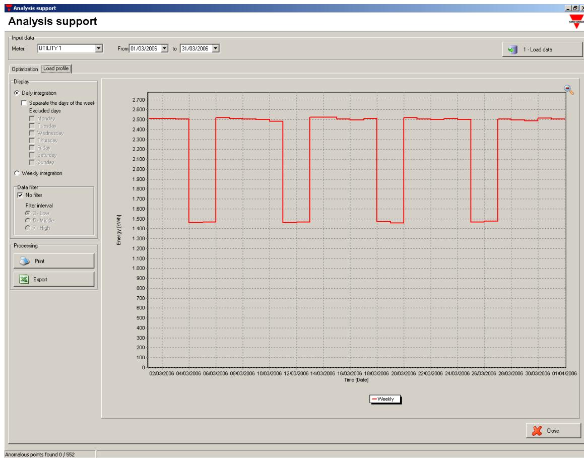
In the database some anomalous data could be present. They can be due to temporary problems of the instrumentation, of the network, of the monitored system or plant: those measurements are real but they can affect the statistical analysis. It is possible to filter these anomalies to get a more homogeneous set of data.
