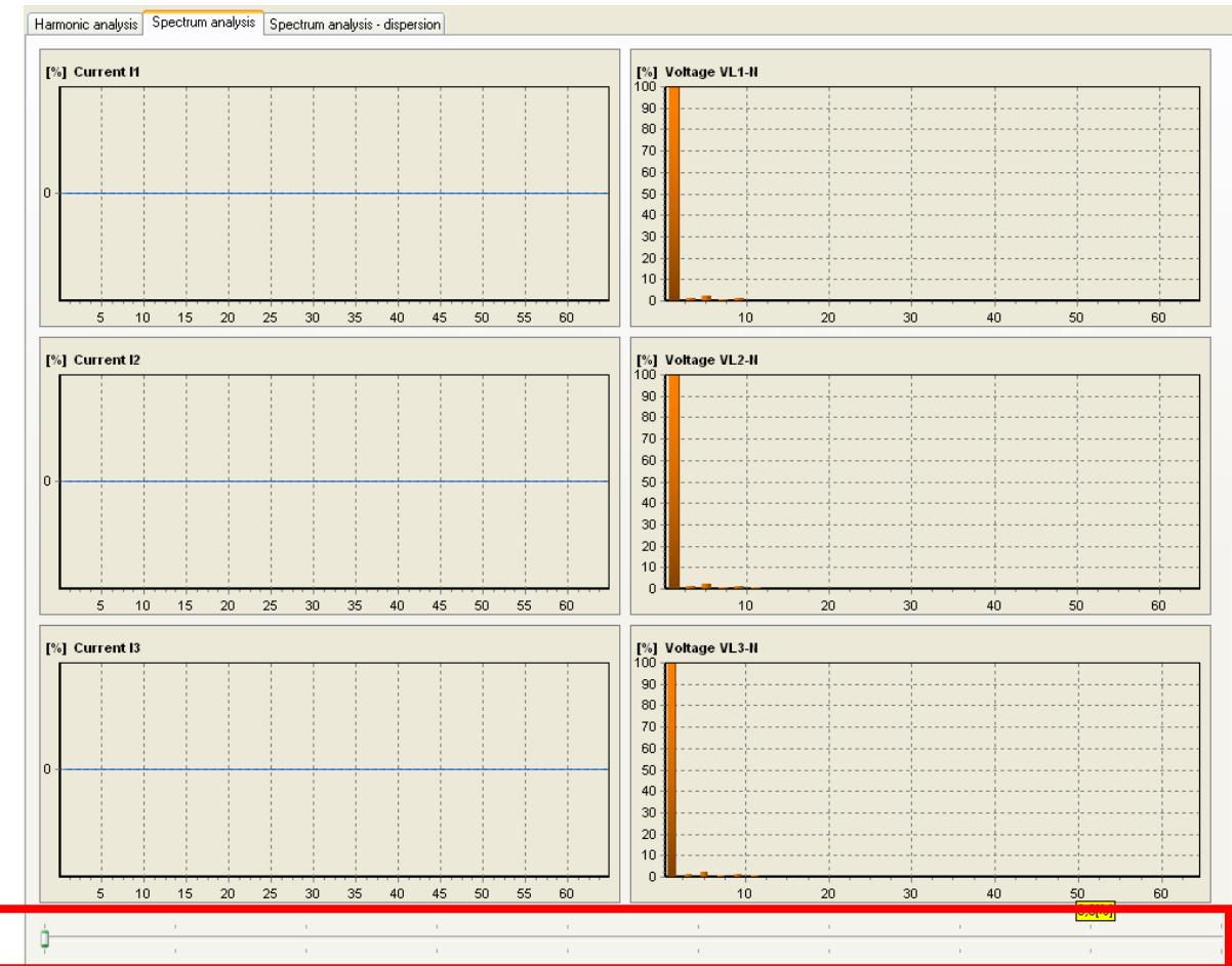
In this section is showed the spectrum analysis for each current and voltage in the frequency domain.
