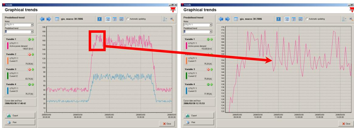
To return back to the original graph, press the unzoom button on the very right of the tool bar.
