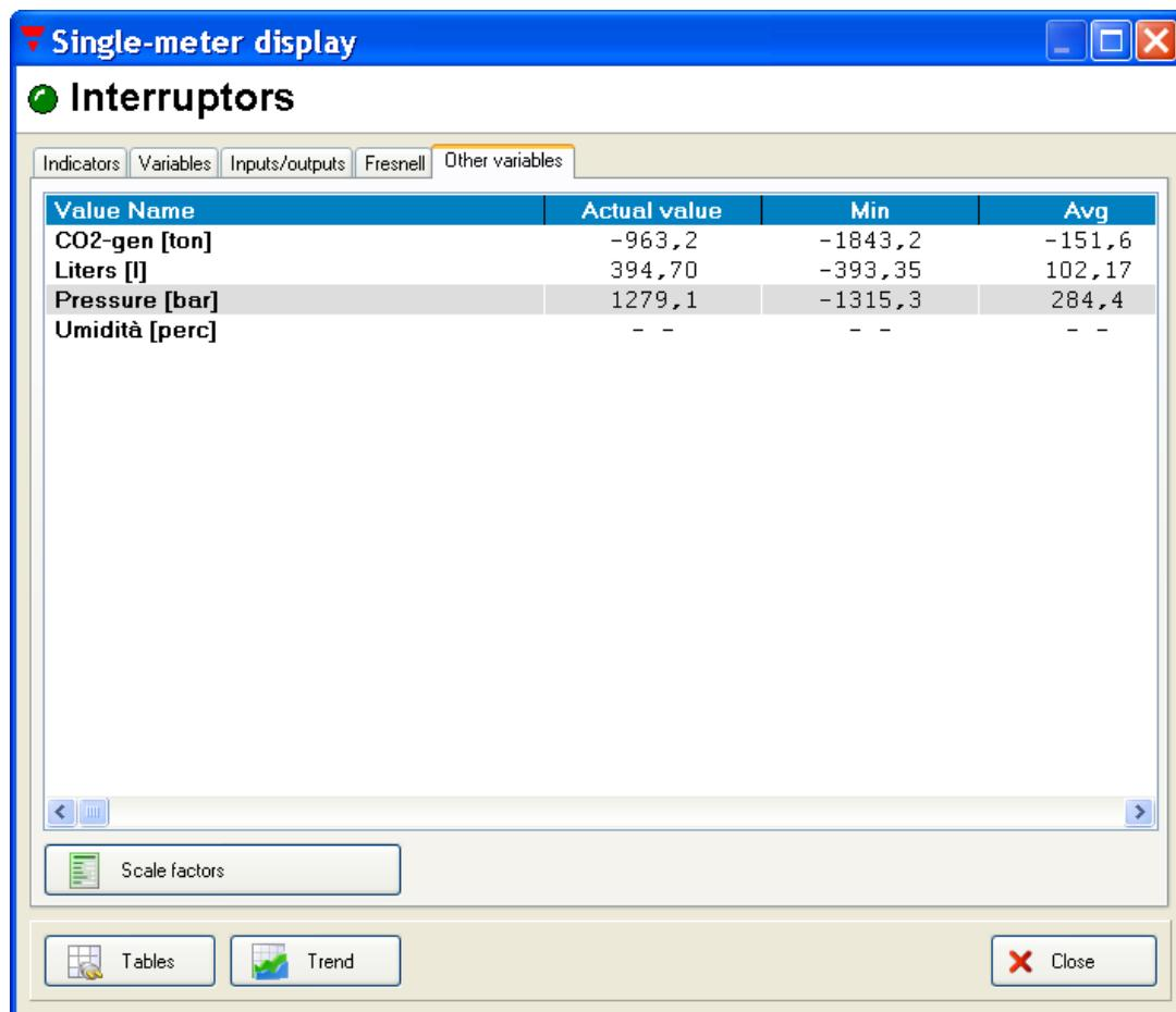
The last real-time value, the minimum, maximum and average values calculated from the last recording are available as per the standard electrical variables.
