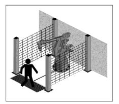
Safety module along with the SM-.. safety mat constitutes a safety system of safety category 3 in conformity with EN 954-1 and can be effectively used for a large number of monitoring exigencies also in harsh environments.
