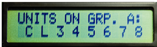
Fig. 57: Offset spaces in slave mode
