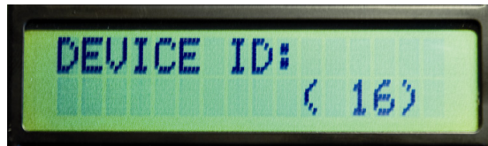
Fig. 51: Device ID for slave mode
