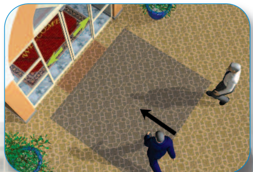
Uni-directional; Doors open only on approach
